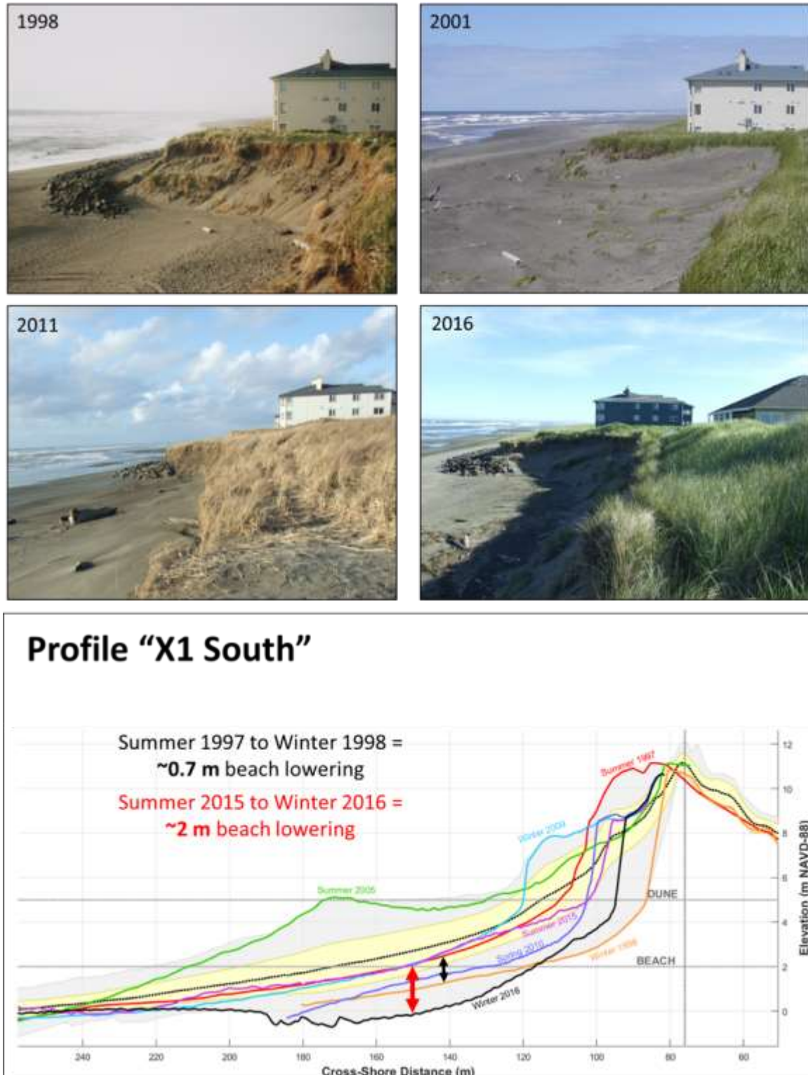
Figure 7-17 Cross-shore Beach Profile Data North of the Ocean Shores North Jetty
