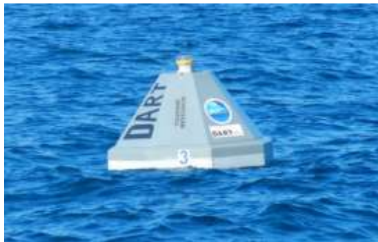
Figure 11-12 Deep-Ocean Assessment and Reporting of Tsunamis System (DART)
